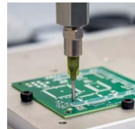
MCT 8040 applied as part of a dam and fill process.
